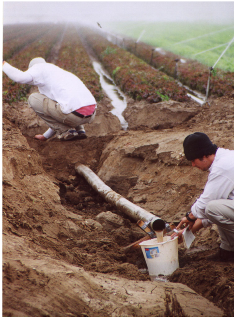
Figure 7.18a. Measuring sediment runoff during sprinkler irrigation. Photo: Fred Watson, 30 June 2000.
