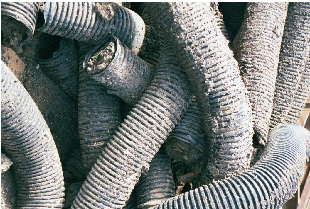
Figure 7.16. Perforated 'tile drainage' pipes removed from beneath a field after clogging up. Photo: Fred Watson, Nov 2001.
