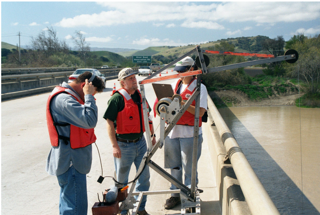
Figure 4.6. USGS field crew measuring an annual peak flow on the Salinas River at Spreckels. Photo: Thor Anderson, 7 March 2001.
