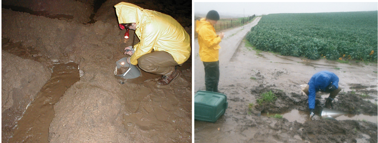
Figure 7.22a. Sampling runoff from agricultural fields during rainfall events. Photos: Don Kozlowski, 19 Feb 2001; Fred Watson, 24 Nov 2001.
